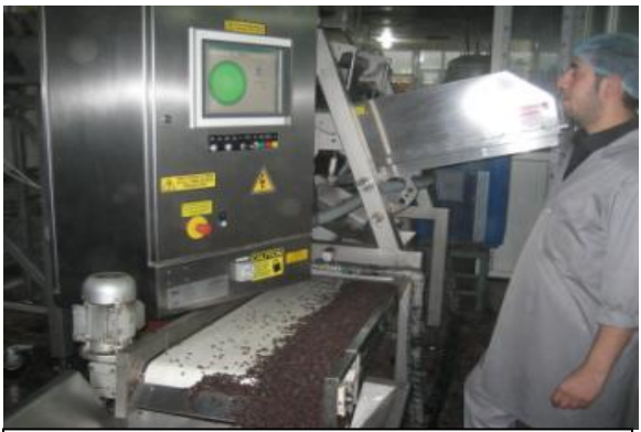
Raisin Processing Industry: Raisin Passing through LASER & X-ray Machines
